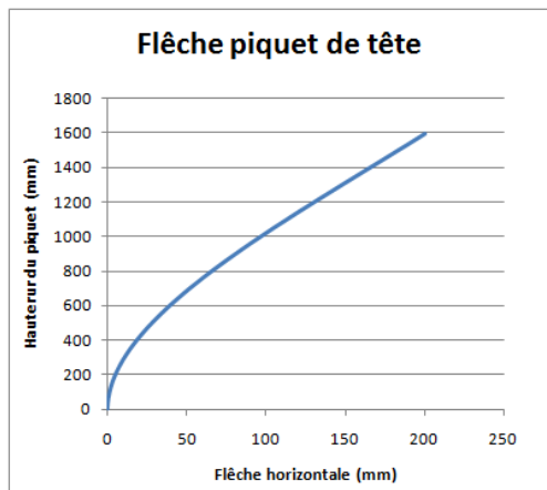
Size adaptatio of the anchored end post to the constraints
